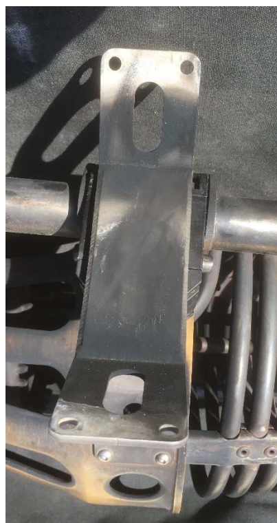
Fig 2. Hanger with doubler plate.
