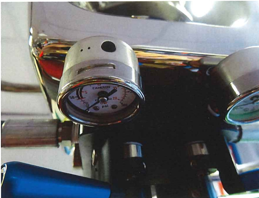
Figure 1. Shadow Single pressure gauge installation
