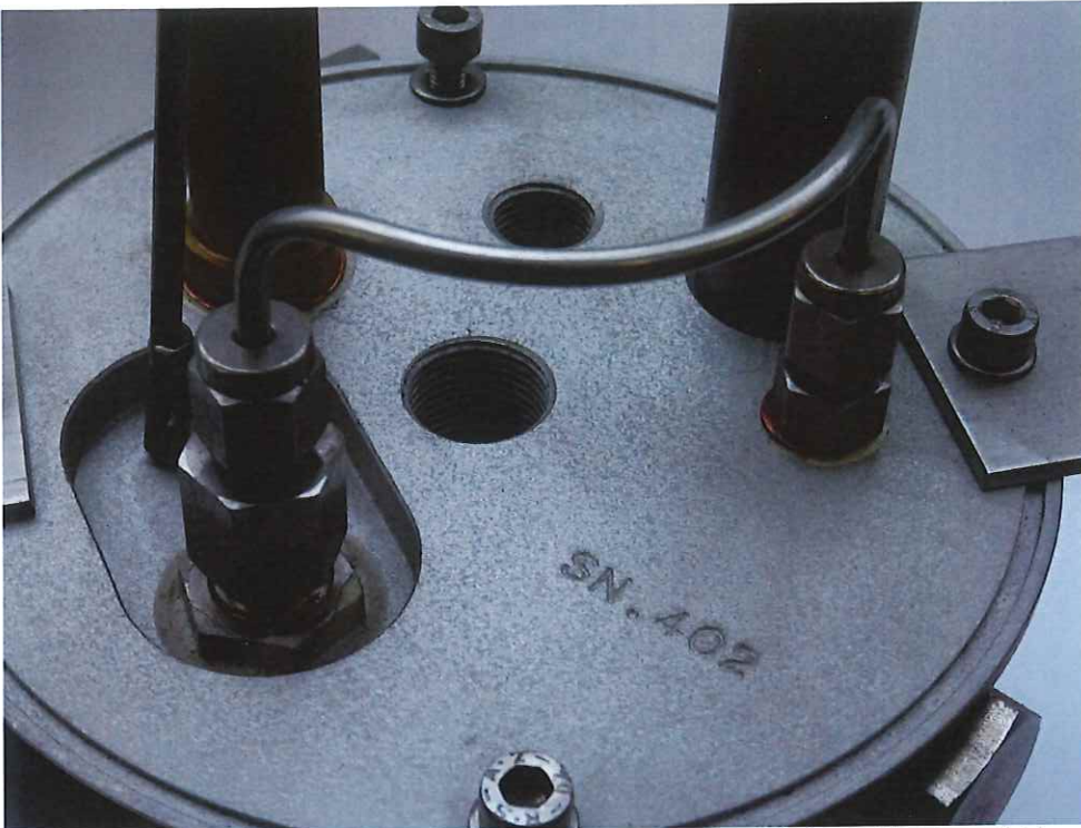
Figure 3. Stratus pressure gauge connection / installation (LH can)
